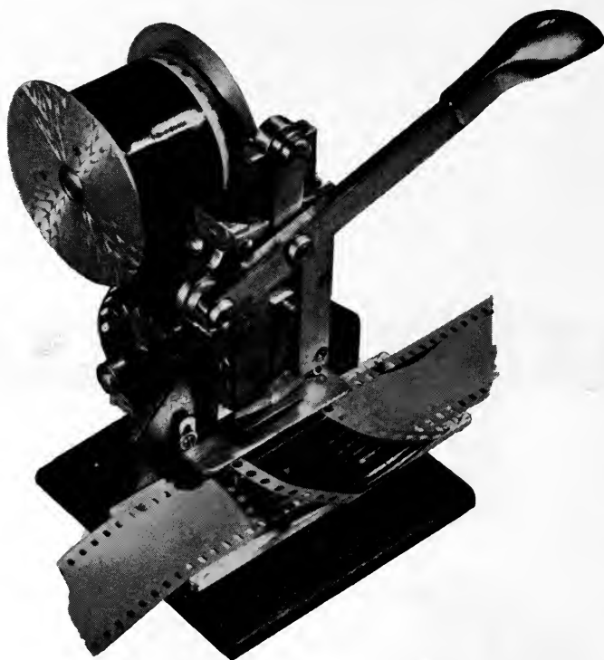
FIG. 11. Machine for utilizing opaque cellophane adhesive.
